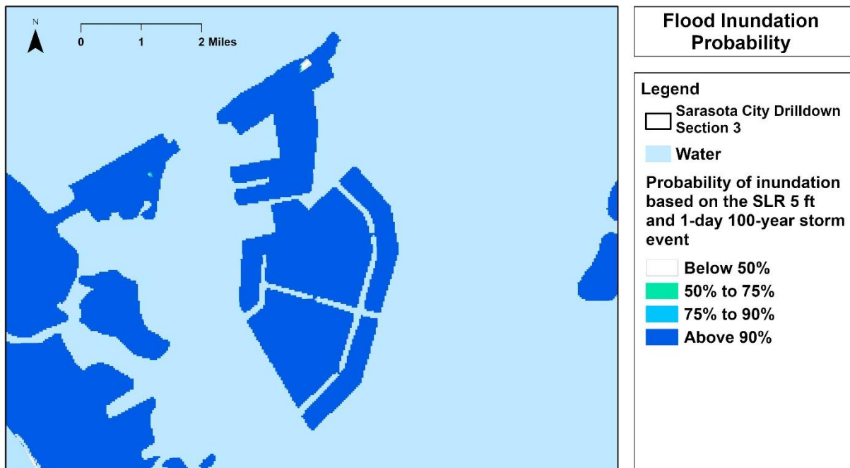
Figure 126. Drilldown of Bird Key, based on 5-ft SLR and 1-day 100-year rainfall event, as generated by FAU CWR3
