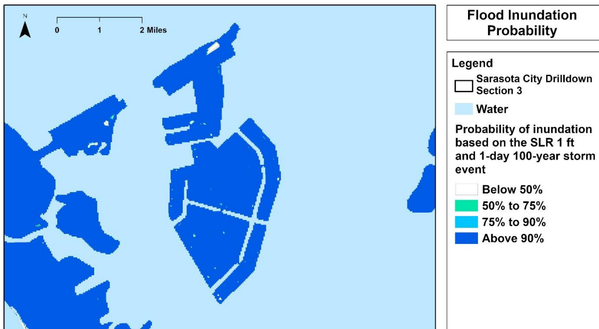
Figure 125. Drilldown of Bird Key, based on 1-ft SLR and 1-day 100-year rainfall event, as generated by FAU CWR3
