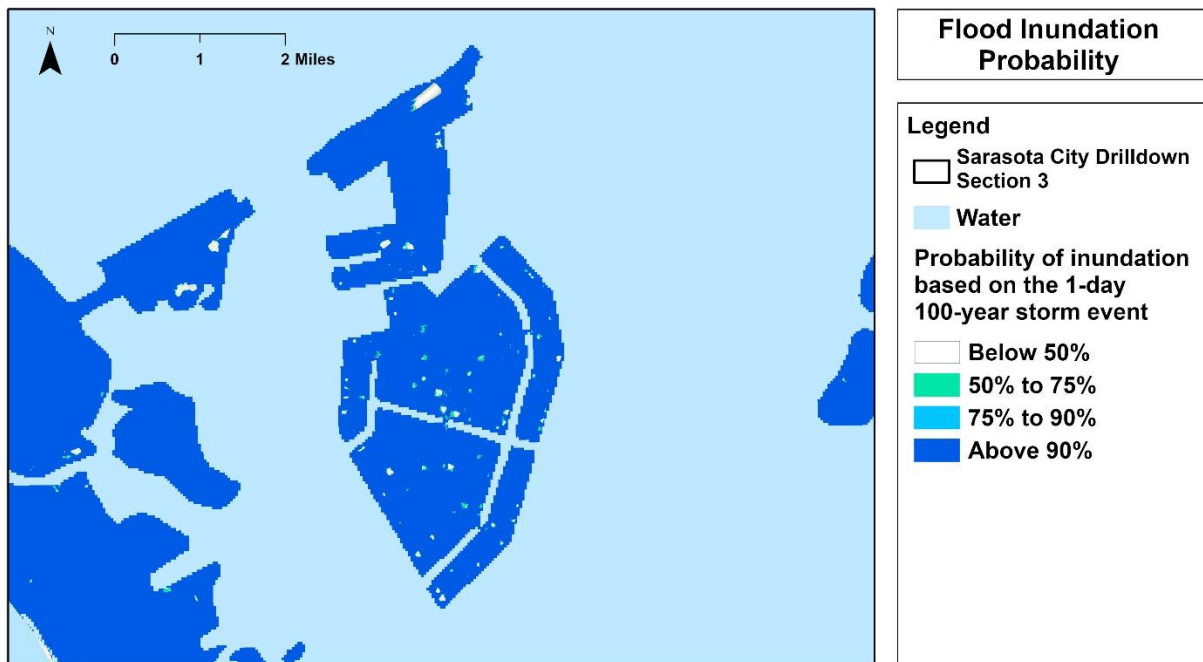
Figure 124. Drilldown of Bird Key, based on 1-day 100-year rainfall event, as generated by FAU CWR3
