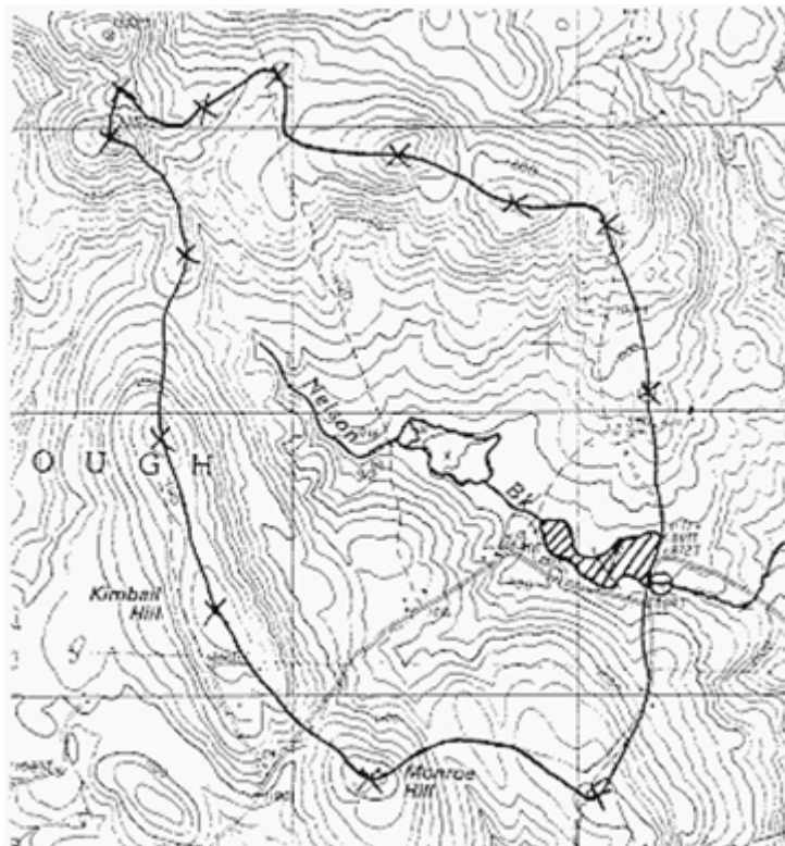
Figure 1. An example of a USGS topographic map used to define a watershed ( https://www.nrcs.usda.gov/Internet/FSE_MEDIA/nrcs144p2_014463.jpg )
